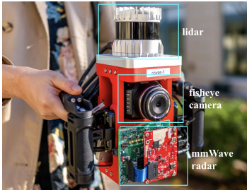
Figure 10. Image of our hand-held data collection rig with three key components labeled.
